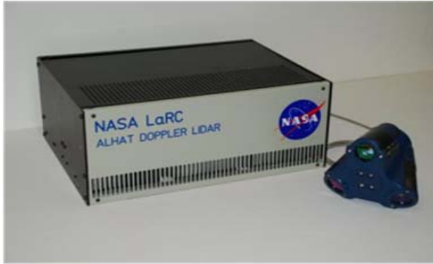
Fig. 3. Doppler Lidar prototype system with a fiber-coupled optical head having 3 lenses pointing to different directions. The Doppler Lidar provides vehicle vector velocity and altitude.
