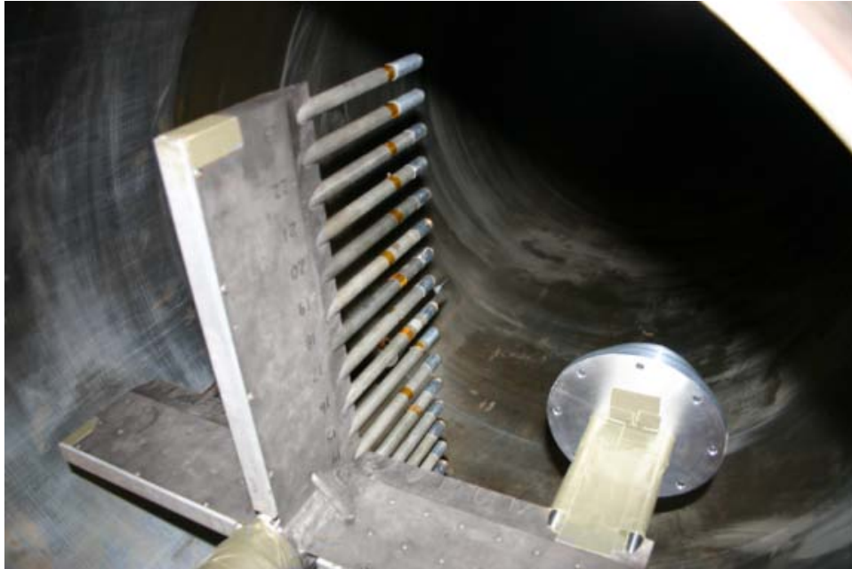
Figure 2, LENS II IH-108 Flow Field Survey Rake
