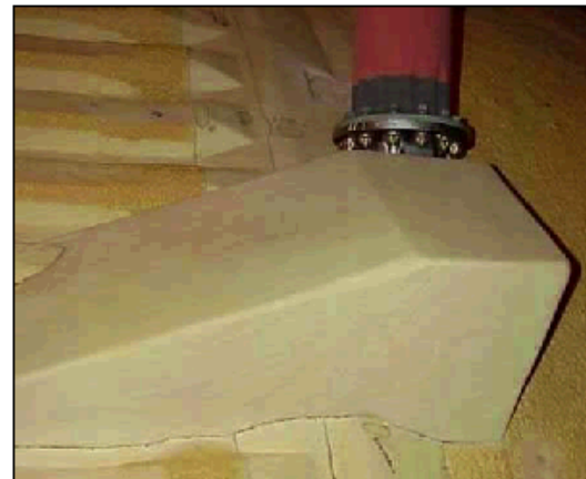
Bipod Ramp (After Final Foam Trim)
