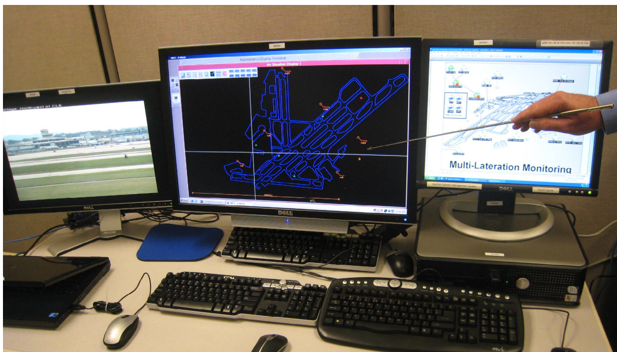
Figure 21.—Multilateration (MLAT) display (center) during AeroMACS communications support.
