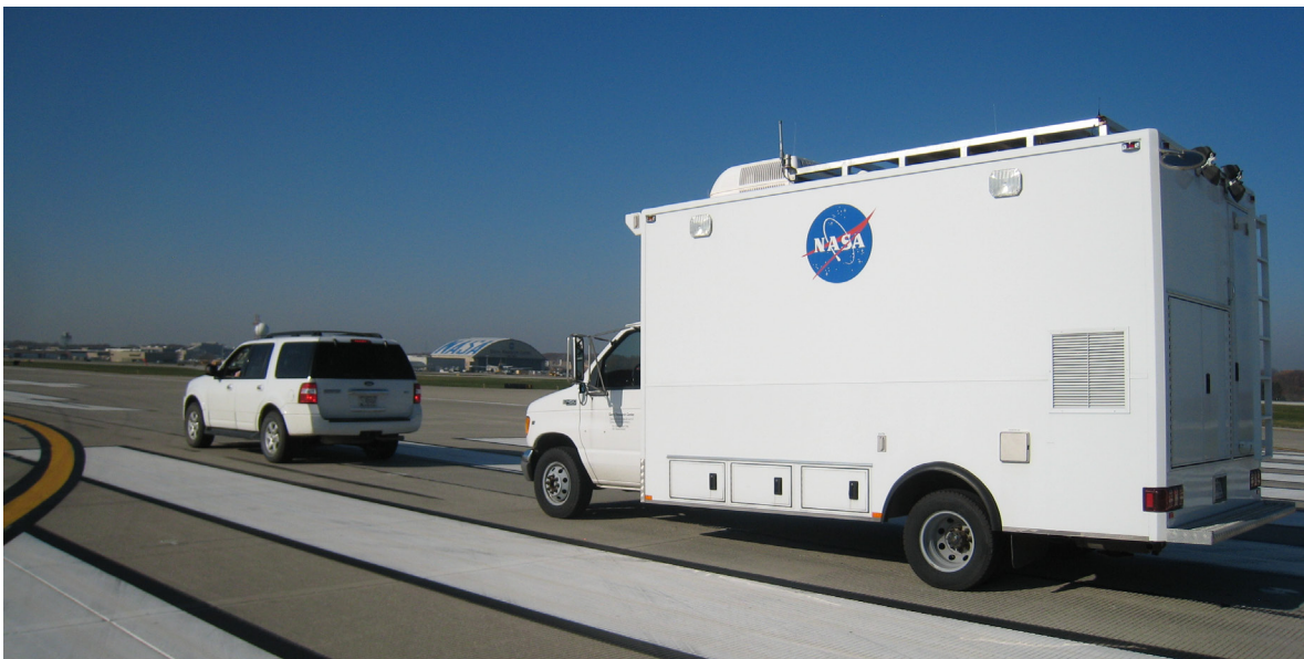
Figure 24.—NASA AeroMACS Research Vehicle (ARV) being escorted by Federal Aviation Administration for mobility tests on CLE airport surface.
