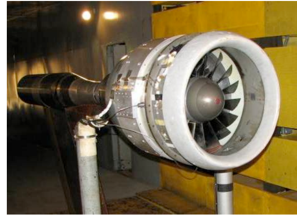
Microwave sensors installed on the NASA Turbofan Test Rig
