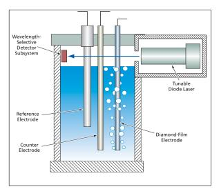
CO2 Would Be Produced by electrochemical oxidation of organic constituents of the aqueous solution, and the concentration of CO2 in the headspace above the solution would be inferred from infrared absorption.
