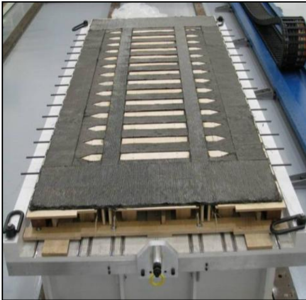
Tear Straps Placed
