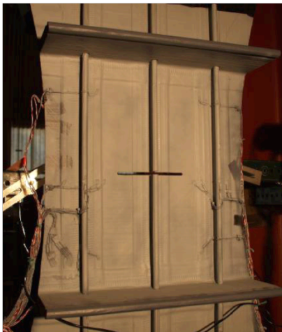
Tension-Loaded Crack-Arrestment Test Panel Baseline
