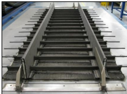
Preform on Mold Tool
