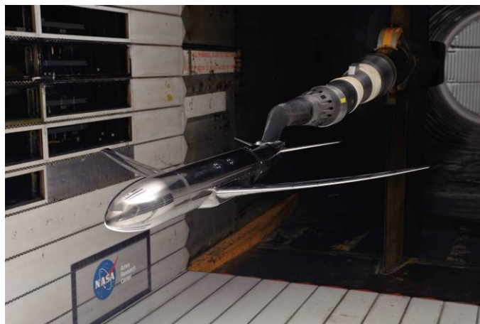
Figure 1. Common Research Model (unpainted) in test section of NASA 11ft wind tunnel.
