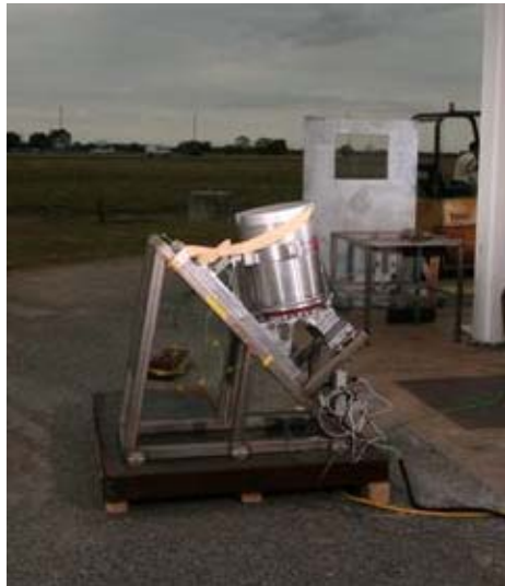
Figure 11 - Drogue Parachute Mortar during Static Firing
