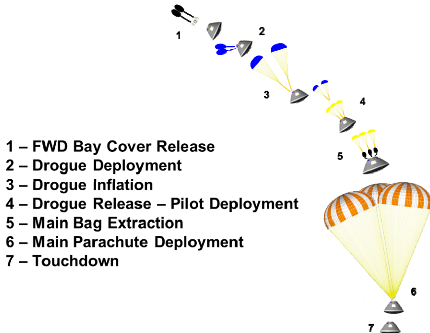
Figure 1 – Basic CPAS/Apollo Parachute Sequence Nominal Entry
