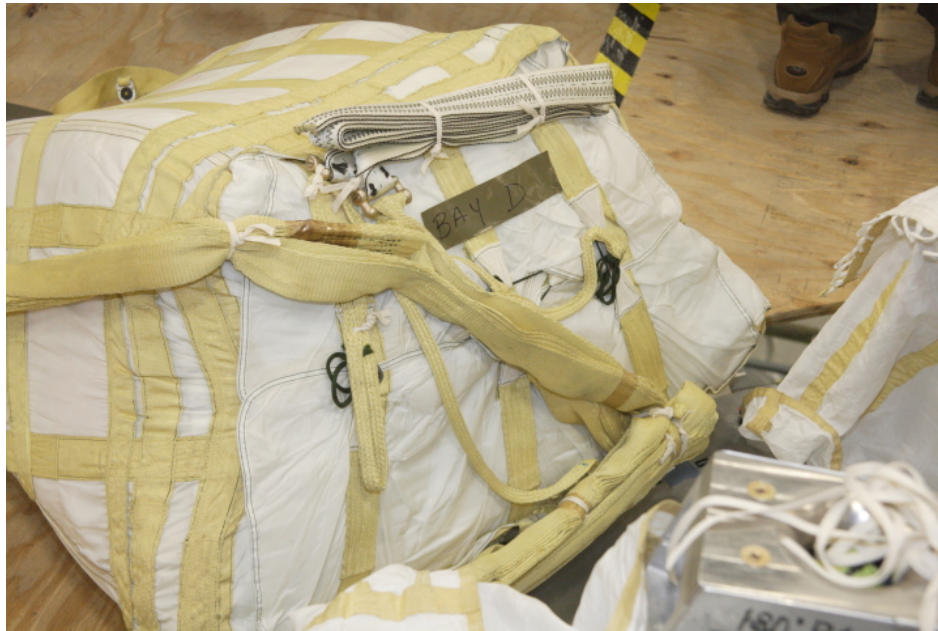
Figure 8 - Main Parachute Confluence Fitting with Attenuators
