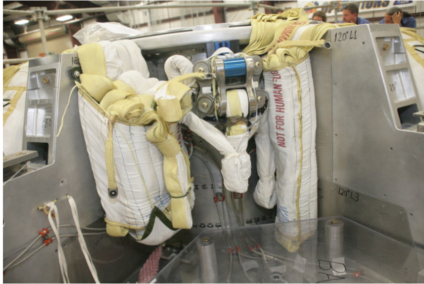
Figure 7 - Main Parachute Confluence Fitting in its Stowage Location.
