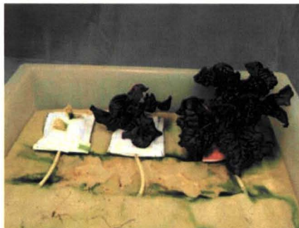
Figure 23. Sustained growth of Outredgeous lettuce in prototype “Rooting Pillows” using Nomex as seed wicking material. Lettuce cv. Outredgeous at 3, 14 and 28 DAP were grown on prototype rooting pillows using an analog root mat using Nomex covered foam was used to perform initial trials.
