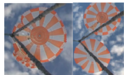
Figure 23. CDT-2-1 full open with a) parachute A crowded out and b) when both parachutes full open.
