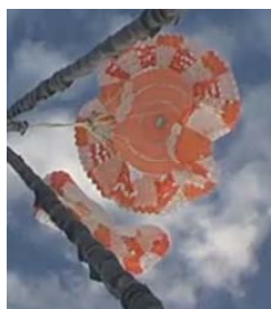
Figure 22. CDT-2-1 second stage disreef.
