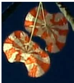
Figure 12. CDT-2-2 second stage disreef.
