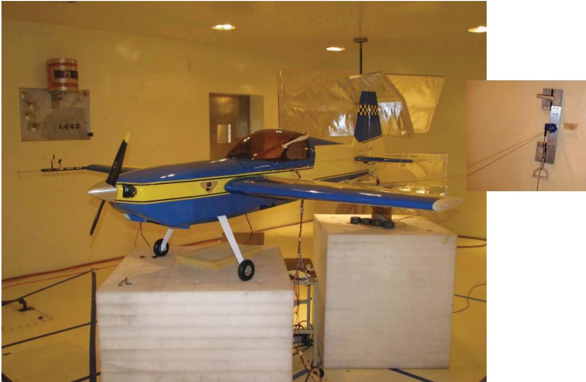
Figure 1: Photograph of the NASA EDGE 540-R2 in reverberation chamber. Also shown (right-inset) is a load cell attached to the chamber wall, for measuring aircraft thrust.
