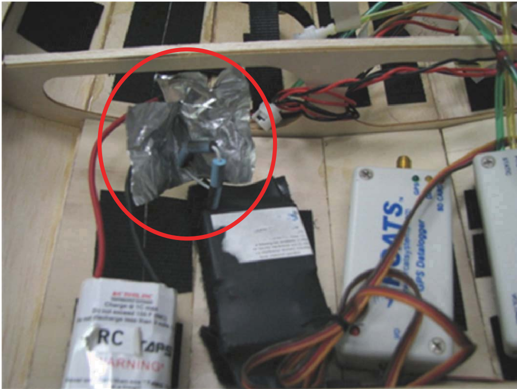
Figure 13: Photograph of ferrite beads and aluminum tape before wrapping over airplane RCATS transmit antenna wire (circled in red) inside NASA EDGE 540. De-tuning the RCATS transmit antenna in this manner allowed better sensitivity for radiated emission measurements.
