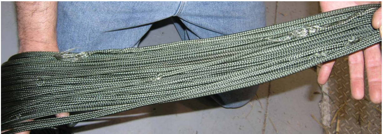
Figure 24. Example of suspension line damage sustained by two drop test main chutes.
