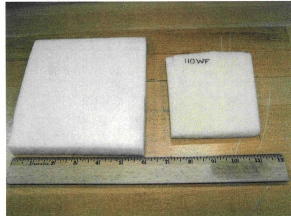
Figure 2: Two samples of 110 WF Rohacell Foam were vacuum dried and subjected to moisture uptake testing in an environmental chamber.
