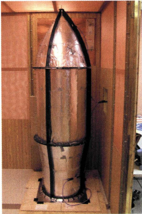
Figure 1. Scaled Fairing Plexiglas Model with Aluminum Foil
