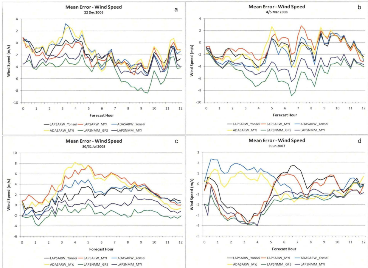
Figure 12. Chart of the mean error for wind speed from the six WRF model configurations for the 12-hour forecast period for a) 22 December 2006, b) 4/5 March 2008, c) 30 July 2008, and d) 9 June 2007.
