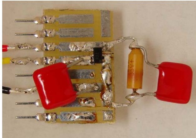
Figure 1. Circuit board populated with ADR3430 chip, input-bypass and output capacitors.
