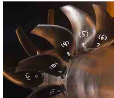
Historical Baseline Blade Set 12 x 10 blade count Non-proprietary geometry/data Export controlled
