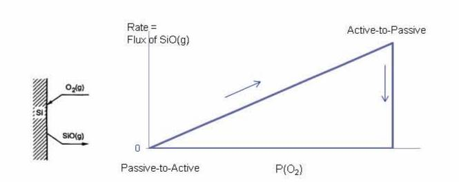
Generate sufficient SiO(g) from reaction (a) for stable Si/SiO<sub>2</sub> equilibrium reaction (b)
