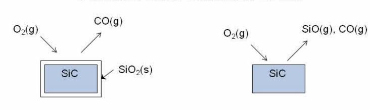
Passive Oxidation [1]  $SiC + 3/2 O_2(g) = SiO_2(c) + CO(g)$  $SiC + O_2(g) = SiO(g) + CO(g)$
