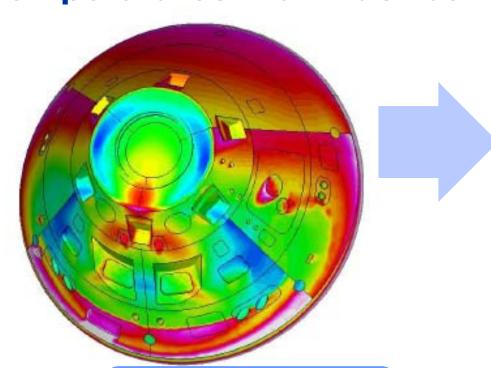
The Orion thermal protection system surfaces can be heated by the reentry plasma to temperatures above 1000 °K creating thermal gradients of several 100 °K over their thickness
