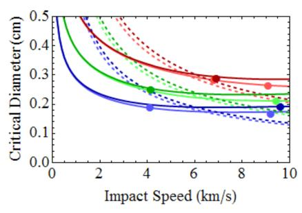
Predicted risk associated with this model relative to an energy scaled model is 60% lower for orbital debris and 95% lower for meteoroids at ISS orbital parameters
