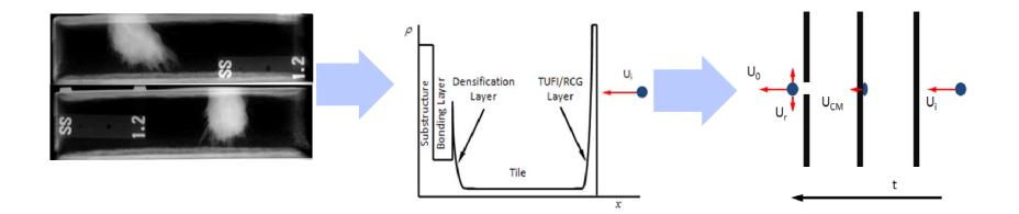
Projectile impacts the higher density TUFI/RCG layer and creates a cavity as it goes through the lower density tile
