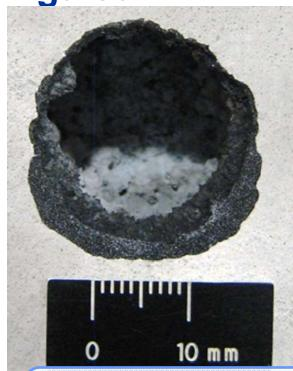
The small dimensions of high probability impacts afford some damage tolerance due to limited thermal convection in the small cavities leaving the residual insulation as the key performance parameter
