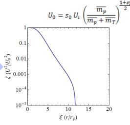
The disrupted projectile expands as it traverses the tile scattering increasing mass to slow faster than a fully intact projectile does  The nondimensional Lagrangian form of the mass, EOS and momentum equations (see Appendix of accompanying paper for full derivation)  The normalized equation for projectile velocity decreases rapidly under expansion until the strength of the tile finally arrests the projectile
