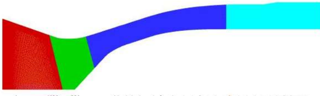
Figure 6: Grid System for Entire UPWT with Test Section 1 at Mach 1.6
