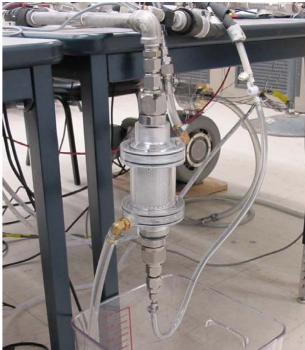
Figure 3. Custom Humidifier Test Configuration.
