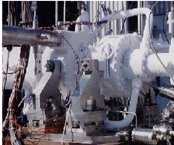
Figure 5: SIMPLEX turbopump (chilled down prior to testing) (Courtesy of NASA MSFC)
