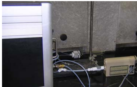
Figure 4. A Commercial DMS was used for initial testing. The Kintek oven is shown on the left and the DMS is on the right. Both devices are placed under the hood.
