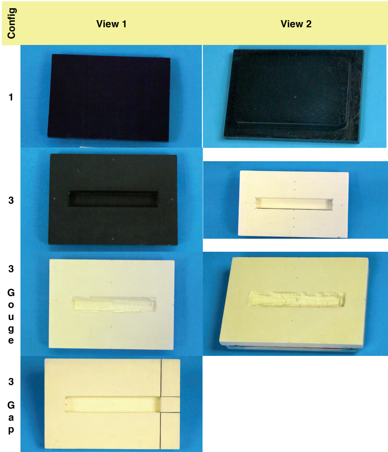
Figure 11. – Cavity insert photographs for Test 6857.
