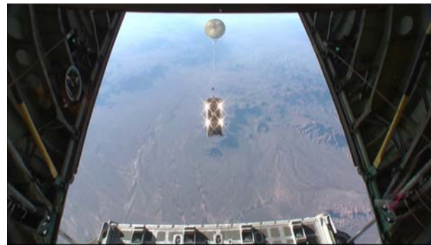
Figure 13. EDU-A-TSE-01C Smart Release trigger. Four flash bulbs mounted on the test vehicle were fired by the avionics system when the release condition was sensed.
