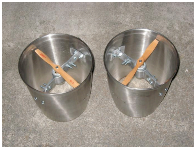
Fig. 5 – Fan & Electric Motor Installation in the Ducts
