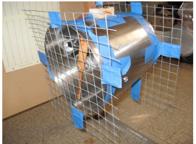
Fig. 8 – Simple Application of Wire Screens (Large Mesh Screen Shown) to Duct Inlet and Exhaust during Static Thrust Testing
