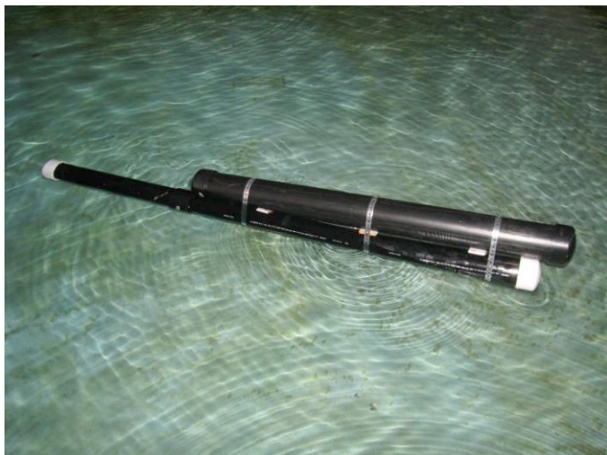
Fig. 13 – Partial Assembly Buoyancy Check
