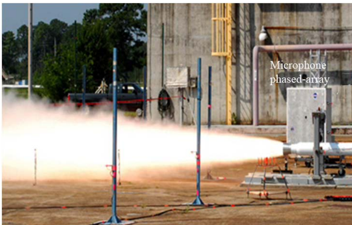
Fig 5. Phased-array during a solid motor firing in a horizontal test stand.
