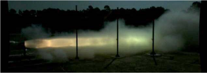
Fig 6. Photograph of the plume by the camera at the center of the phased-array plate.
