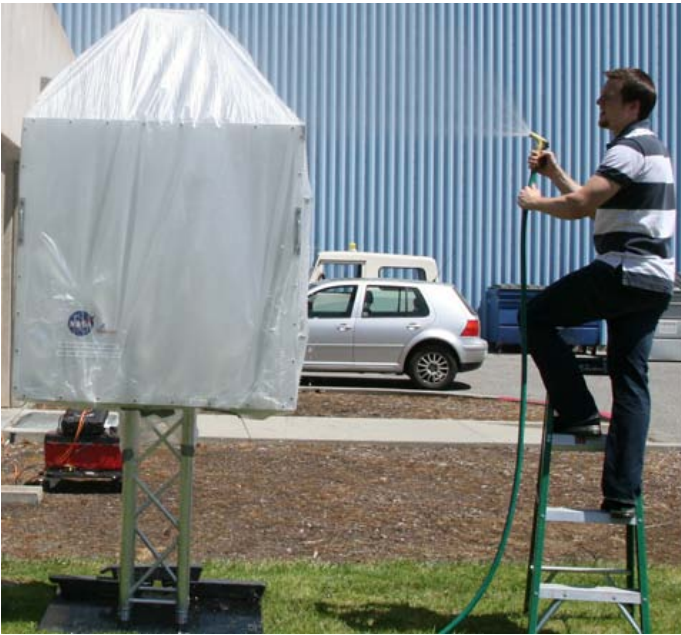
Fig. 2(a) Simulated rain test on the environment chamber (covered by a plastic wrap) at NASA ARC to verify water-proofing.
