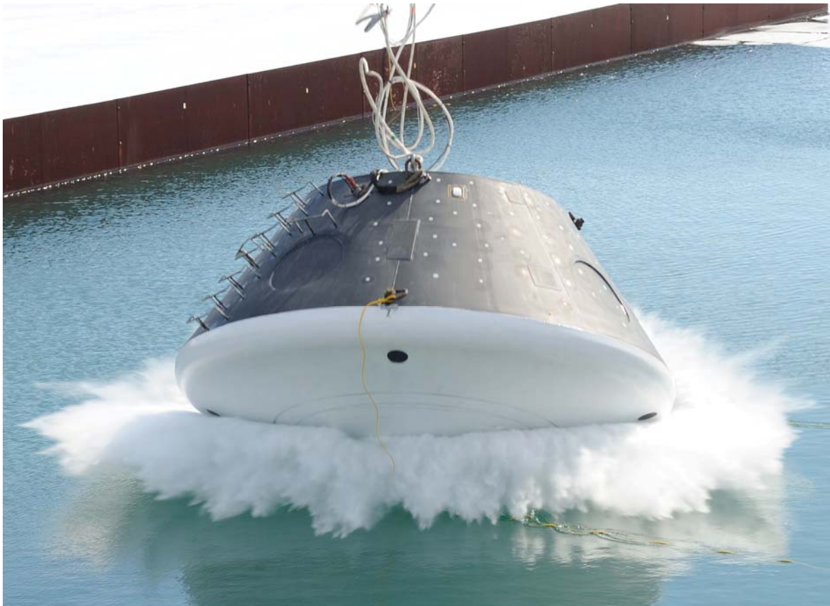
Figure 6. Orion CM boilerplate water drop test at Aberdeen Proving Ground.
