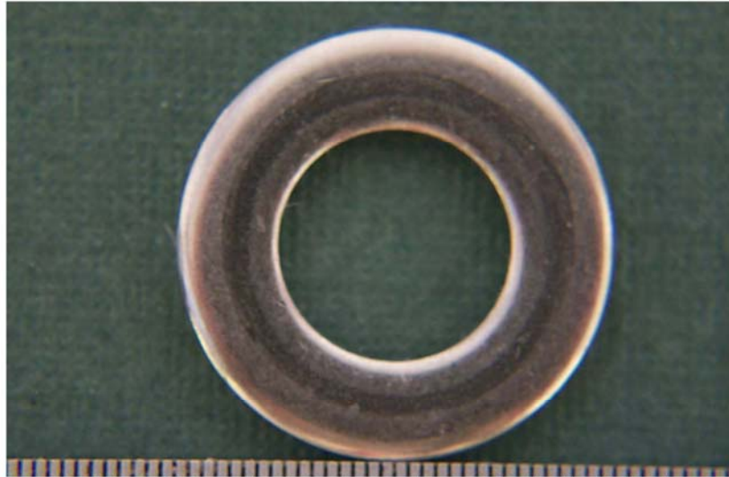
Figure B4 Top side of a washer used "as received" without cleaning.
