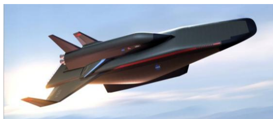
Figure 3. Two-stage-to-orbit launch vehicle concept with a turbine-based combined cycle first stage and a reusable, rocket-powered second stage.
