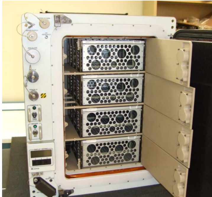
Figure 4. Glacier with door open showing regular size trays
