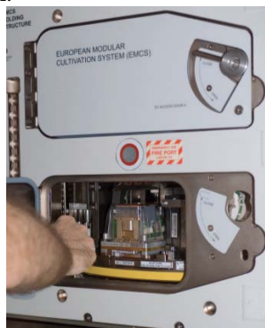
Figure 3 ISS crewmember replacing the European Modular Cultivation System (EMCS) Experiment Container (EC) in the Destiny laboratory of the International Space Station. Image courtesy of NASA.
