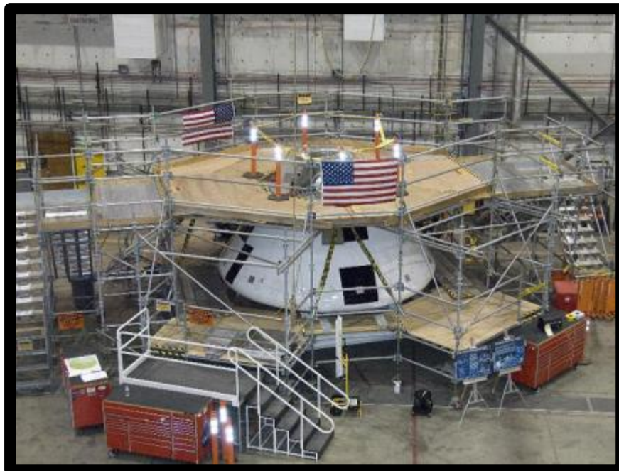
Crew Module being integrated in Shuttle Hangar at NASA Dryden Flight Research Center
