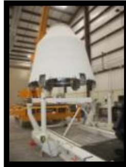
Adapter Cone placement
