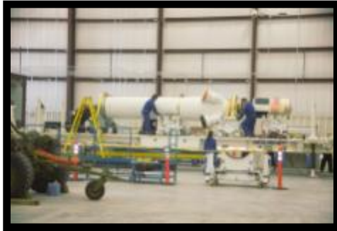
Motor Roll Transfer onto integration trailer
