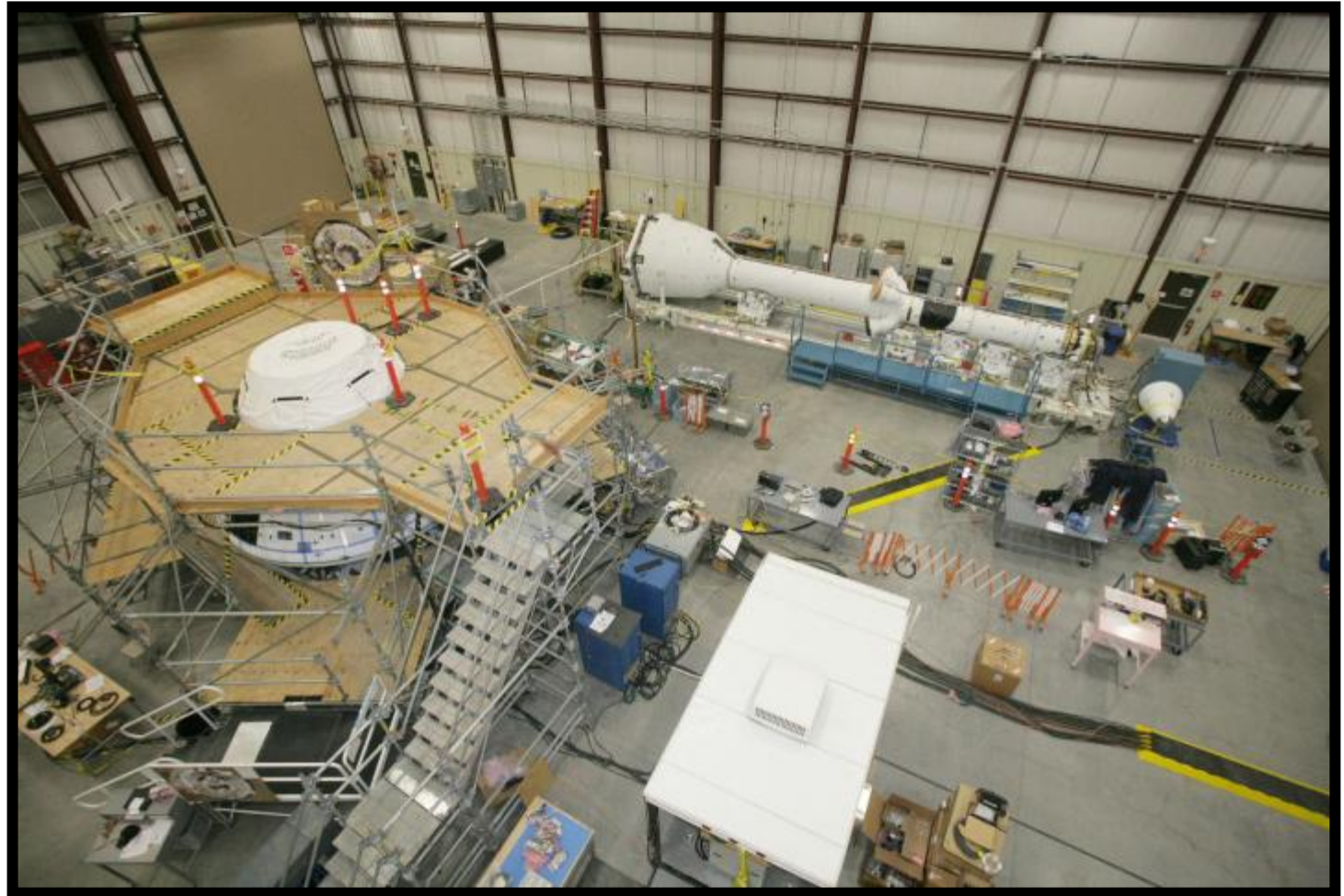
Crew Module / Launch Abort System Soft Mate Testing
