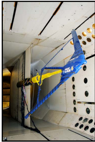
Figure 1. JWS model in TDT in aft sting mount test configuration, Test 606
