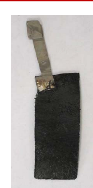
Figure 8 Free standing carbon-silicon nanofoam anode
