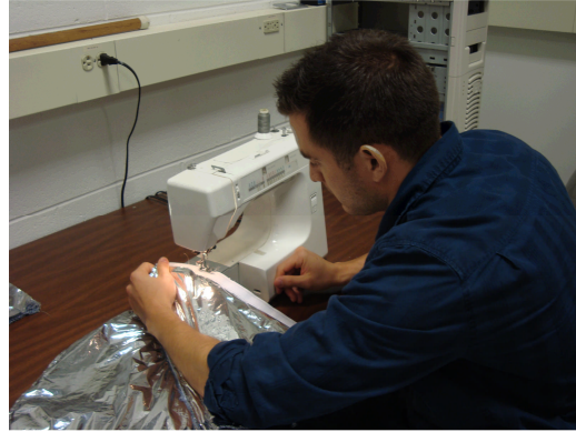
Figure 8. Sewing of MLI blanket sections
