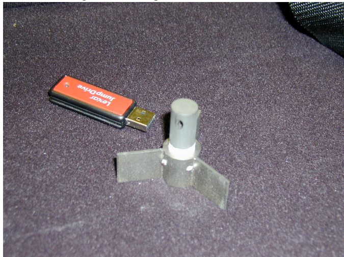
Figure 3. CERMET specimen with black body cavity.
