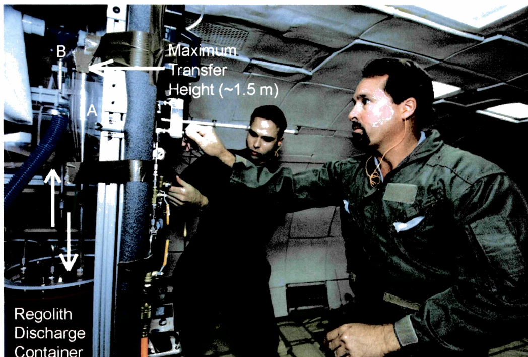
Figure 3. Photo of the RGF experiment showing Tephra that fell from cyclone A into the Regolith Discharge Container. The Tephra flowed vertically upward along a convey pipe from the eductor located at the bottom of the Supply Container (not visible in photo). The convey pipe had a vertical-to-horizontal transition which connected it to the inlet of cyclone A. The gas exhaust from cyclone A became the input for the smaller cyclone B, which discharged dust into the blue hose shown in the picture. The exhaust from cyclone B passed through HEPA filter bags before exiting into the transparent containment box, which had a secondary HEPA filter that allowed the filtered air to enter into the aircraft cabin.
