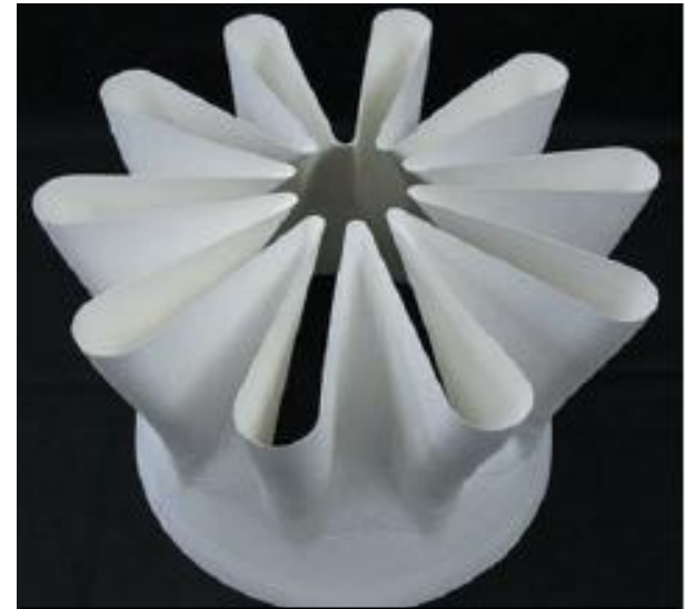
18-inch dia. CMC Mixer Demonstration Article
