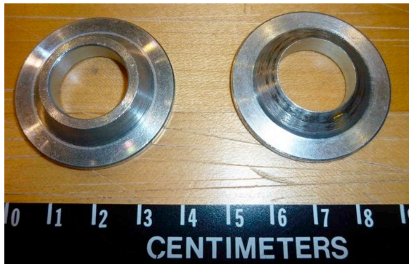
Figure 17. Conical washers (left - original; right - modified).
