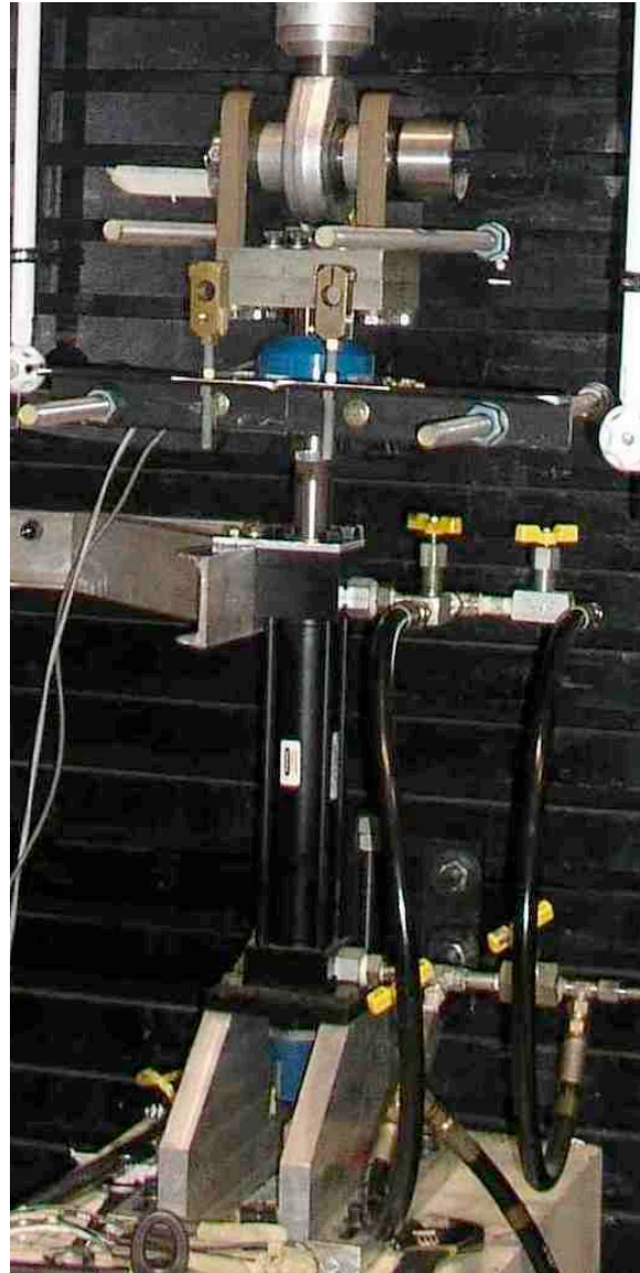
Figure 9. Hand-operated hydraulic actuator for lightly loaded strut tests.
