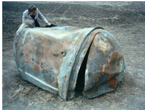
Figure 1. A 250 kg., stainless steel Delta 2 second stage reentered and landed in Texas in 1997.
