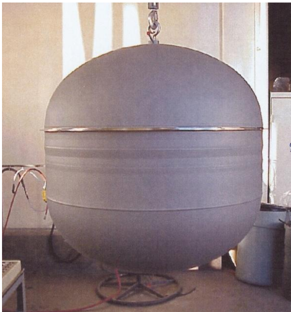
Figure 3. Titanium fuel tank design used for the USA-193 spacecraft.
