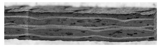
SEM of RTM370 made by VARTM Void content = ~6.5% after postcured at 650°F/8 h Resin=35-38 wt%, Fiber volume=49-53%
