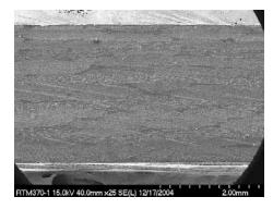
RTM370 Made by RTM Void content= ~1% Resin = 35-36 wt% Fiber volume=53-56%
