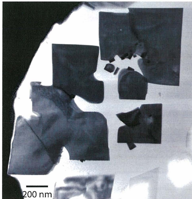
Figure 4. Bright Field TEM image of mullite crystals with a skeletal morphology, indicative of rapid crystallization from a silicate melt.
