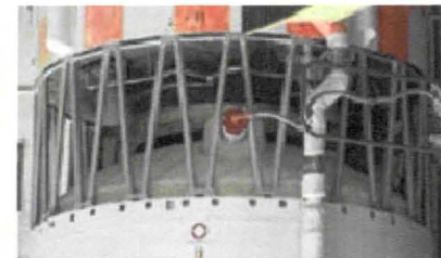
Open compartment inter-stage design with concentric-nested upper stage
