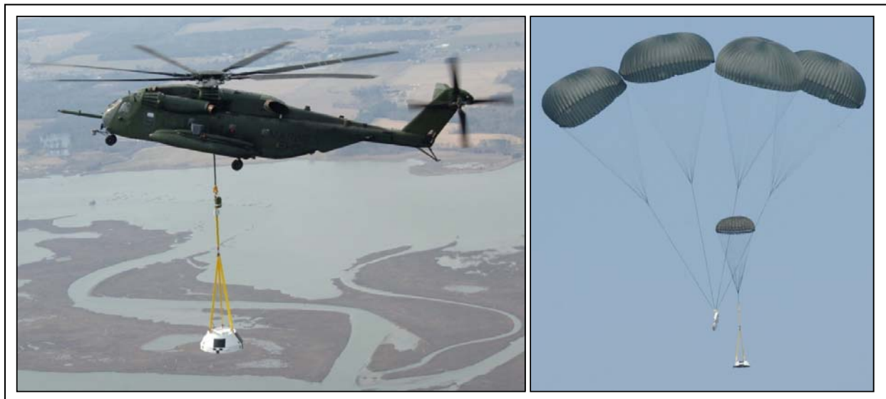
Figure 9: LPD drop test.
