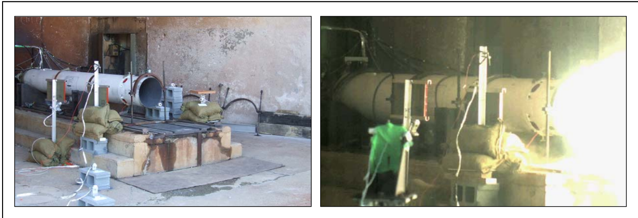
Figure 10: Static rocket motor firing to collect thrust, thermal, and acoustic data from similar age motor.
