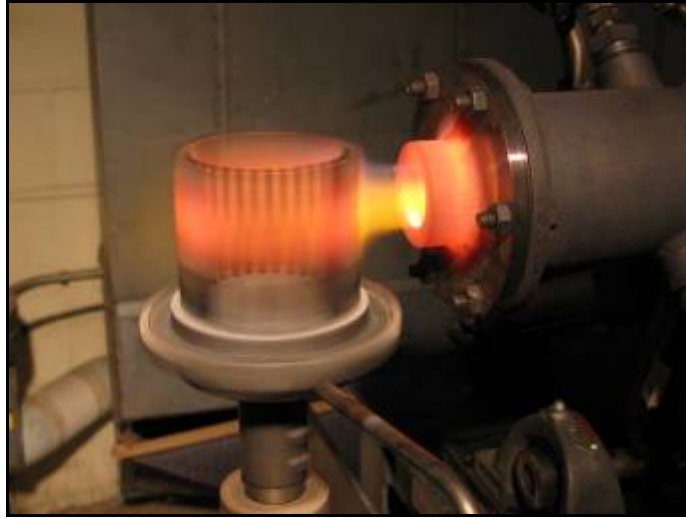
Figure 9.—Carousel holding eighteen specimens, each 1/4 diameter by 3 in. tall. Samples were undergoing synthetic sea salt corrosion to determine the effectiveness of protective metallic coatings.
