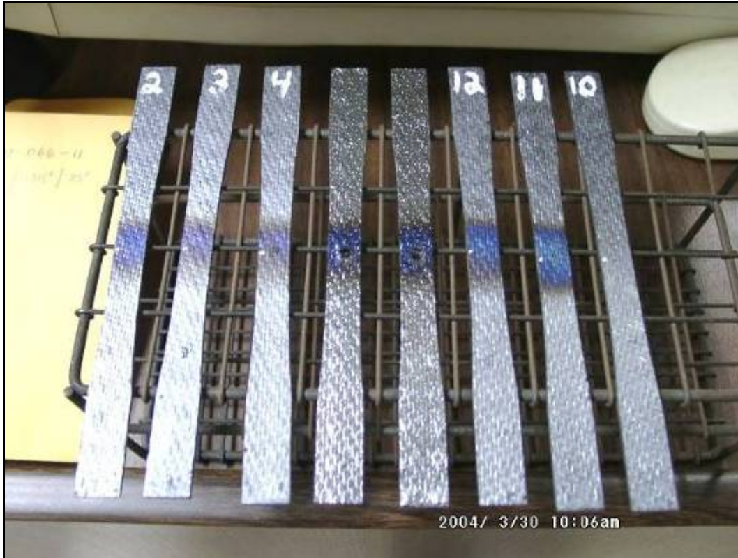
Figure 12.—Uncoated CMC tensile “dogbone” specimens (6 by 1/2 by 1/8 in.) after impact with a 1/16 in. diameter steel ball bearing at various temperatures and projectile velocities.
