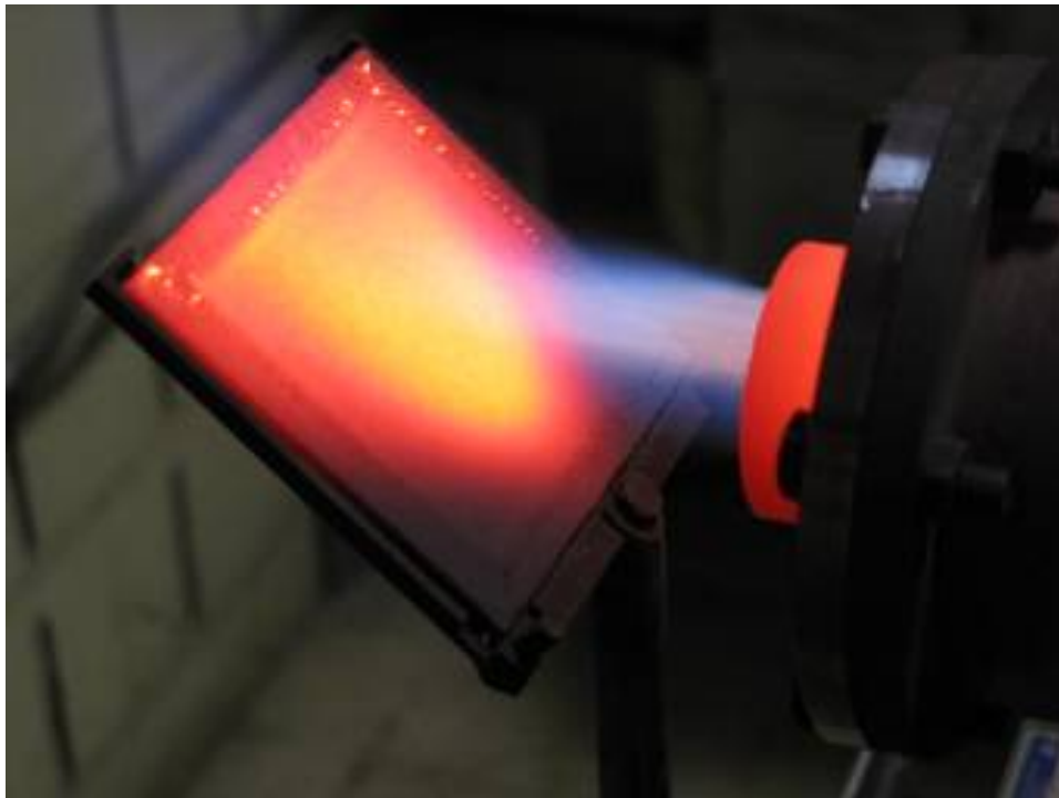
Figure 7.—Durability testing of a 3 by 3 in. superalloy plate protected with a thermal barrier coating.
