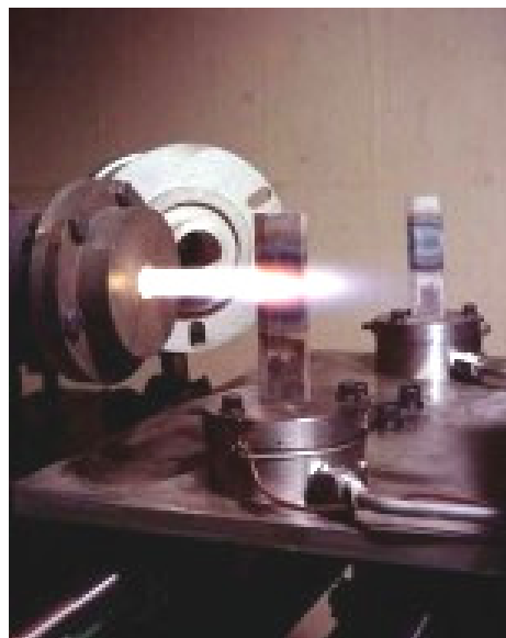
Figure 23.—Mach 1 burner rig. NASA photo C-1977-1605.
