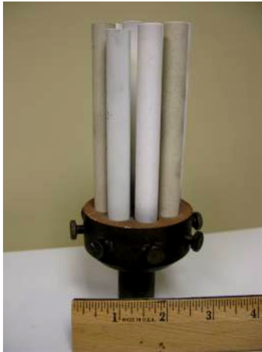
Figure 18.—Eight place carousel for burner rig exposure of a multiple thermal barrier coated superalloy specimens. Nominal size of coated solid rod: 1/2 in. diameter, 5 in. tall.
