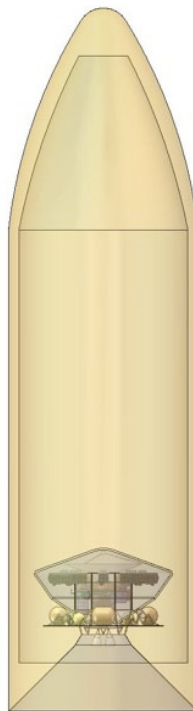
Figure 2.8.—REP Flagship S/C in Delta V payload fairing.
