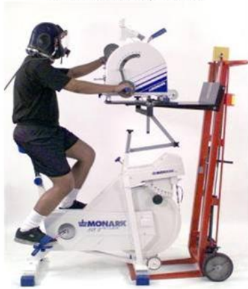
Dual-Cycle Ergometer used for Exercise-Enhanced Prebreathe
