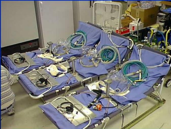
Suit simulator set up for multiple semi-recumbent intermittent light exercise simulating astronaut tasks
