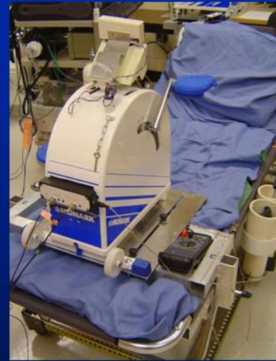
Suit simulator set up for leg ergometry
