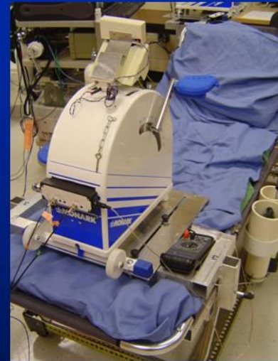
Suit simulator set up for leg ergometry
