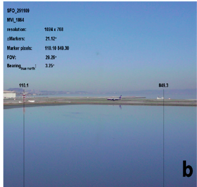
Figure 3. The video field of view used for motion tracking during the braking phase of landing.
