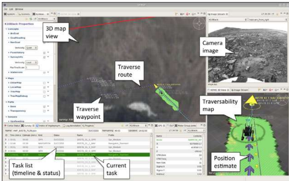
Figure 10. The Visual Environment for Robotic Virtual Exploration” (VERVE) is an interactive 3D user interface for monitoring robot operations.
