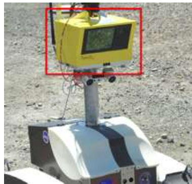
Figure 4. K10 carries a mast-mounted 3D scanning lidar.
