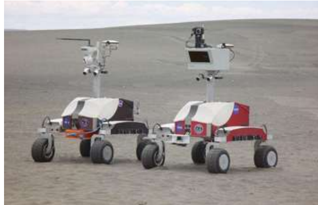
Figure 2. K10 “Black” and “Red” planetary rovers are equipped with a variety of science instruments.
