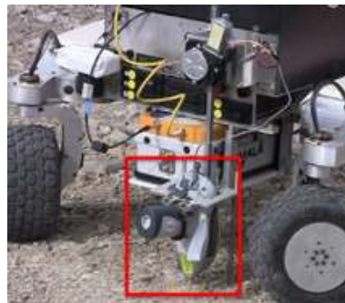
Figure 6. K10 is equipped with a deployable x-ray fluorescence (XRF) spectrometer.
