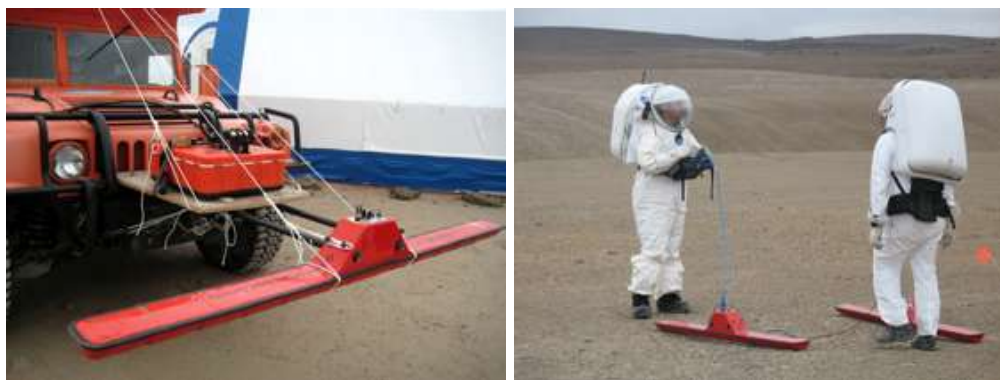
Figure 16. Ground-penetrating radar (GPR) at Haughton Crater. Left, a GPR is mounted on the front of a simulated pressurized crew rover; right, GPR is manually deployed by suited crew.
