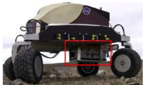
Figure 5. A ground-penetrating radar is mounted underneath K10.
